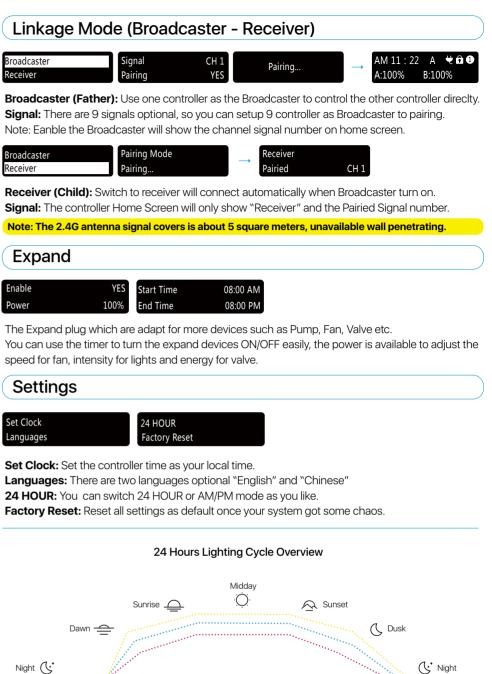
The Control system will gradually ramp the intensity of LED between set points. The graph below outlines how the LEDs will ramp up and down between settings.
