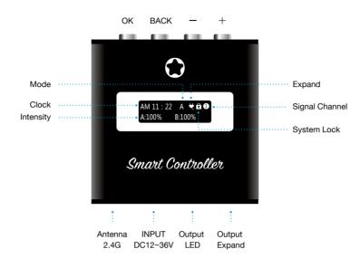
Special Function 1: Hold on "OK" 3 second under locked to switch Auto & Manual Mode quickly. Special Function 2: Hold on "BACK" 3 second to unlock and lock system. Special Function 3: Hold on "OK" + "BACK" turn to the Receiver Mode quickly.
