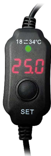
Fig. 1: Controller with temperature display and button for setpoint adjustment
