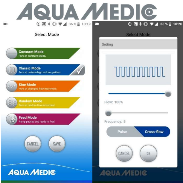
Fig. 26: ... then you tap on the wave symbol in front of "Classic Mode" and select "Cross-flow" (is then highlighted in blue). The pump power is adjusted under "Flow", the switch-on and switch-off time with "Frequency" (minimum approx. 30 seconds, maximum approx. 90 minutes). Save with "OK" and "Save". It can take up to three cycles for the pumps to "find" their alternation rhythm. You should therefore start with a cycle at the lowest level and increase it when the pumps change evenly.
