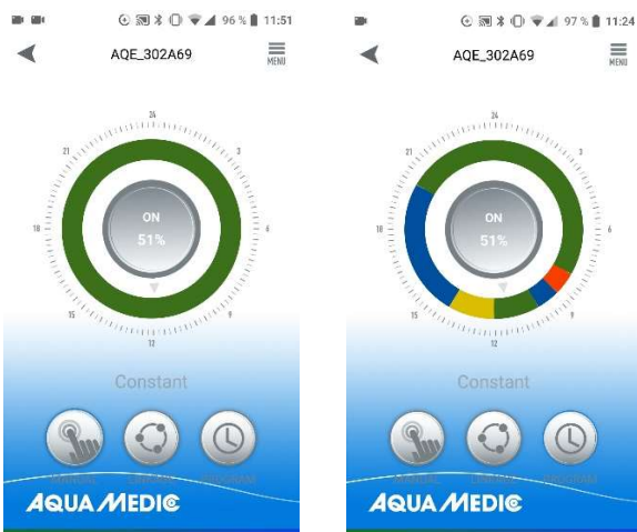
Fig. 19: To activate a program that has been created, the PROGRAM button has to be briefly touched. The display then changes to the created program.
