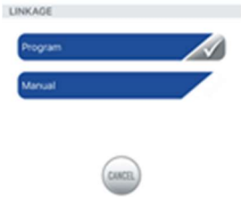
Fig. 21: A program mode or a manual mode can be set for the "MASTER" pump. The setting is made as described under Manual mode or Timer mode.
