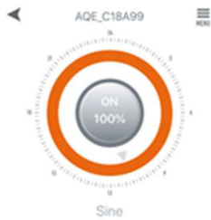
Fig. 27: In the menu at the top right it is possible to rename or delete pumps.
