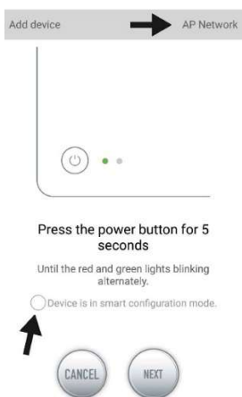
Fig. 4: The desired mode is confirmed by tapping on the circle above the lower arrow. By tapping on "AP Network" or "Smart Network" next to the upper arrow (the arrow is not available in the APP), you can switch between the two modes. (The "Smart Configuration Mode" must be selected here. The green and red LEDs only flash in the case of dosing pumps; in the case of pumps, the blue WiFi symbol flashes in the controller).
