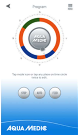
Fig. 10: Touch the "STOP, AUTO, FEED" symbol or double-touch the circle to edit the respective period.
